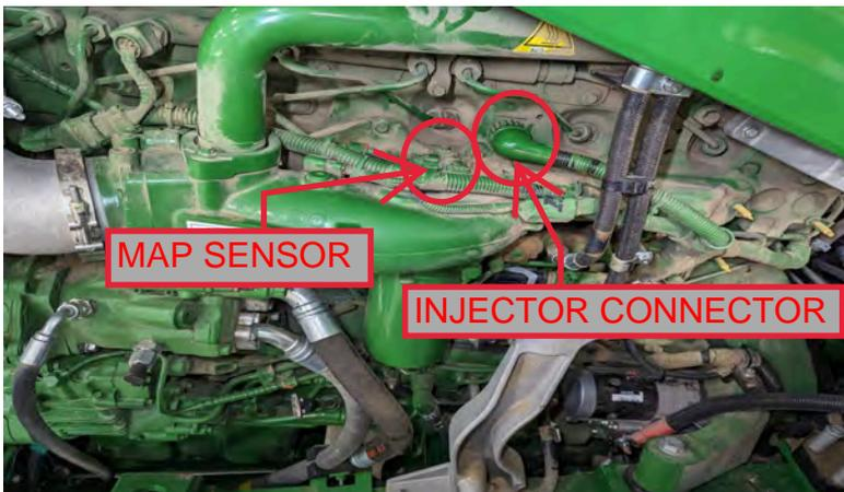
2) Plug male module connector into factory female connector in cylinder head. Plug female module connector into male factory harness connector.
