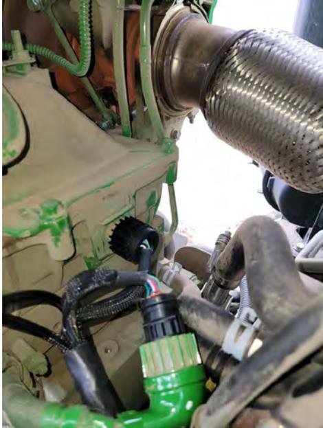
3) Connect the Male MAP Sensor plug from the module into the Stock location and the Stock Male MAP Sensor plug into the Female plug from the Module.
