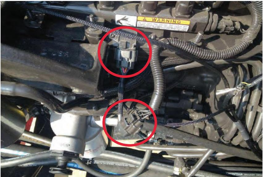
5) Route the red power wire to the alternator, +12 volt constant source. The black wire will connect to a good Ground.
